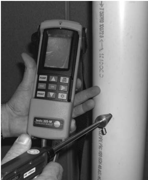
Figure 9.2: Insert Analyzer Test Probe into Test Port
